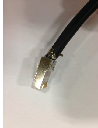
16. Push the external tab inward to the cable. 17. Wrap the drain wire multiple times around the external ground ear tabs.
