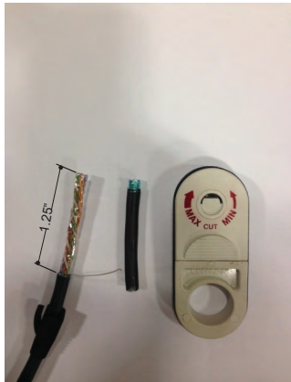
1. Slide Boot (CN-B0051) onto cable 2. Strip the jacket 1.25" to 1.5" 3. Be sure to strip jacket and foil away from the cable.
