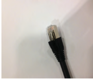
20. Slide the boot over the connector body.
